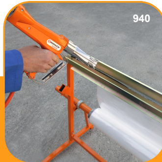
Bag sealing with RIPACK® heat shrink tool *
